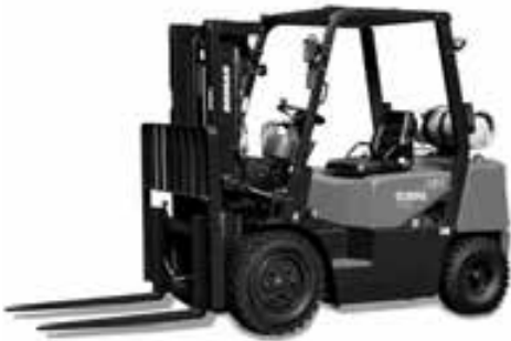
G20G / G25G / G30G 4,000lb 5,000lb 6,000lb LPG, Pneumatic Tire
